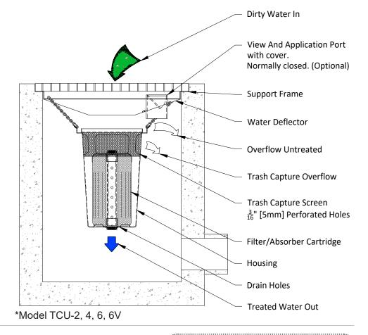
The Water Decontaminator Trash Capture series is engineered and patented for the treatment of stormwater run off. We design our filters to meet or exceed stormwater best management practices (BMP's) and best available technology (BAT).
